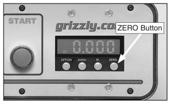
Figure 59. Digital readout zero button.
